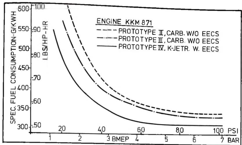
Figure 16. - Specific fuel consumption at 2000 rpm.
