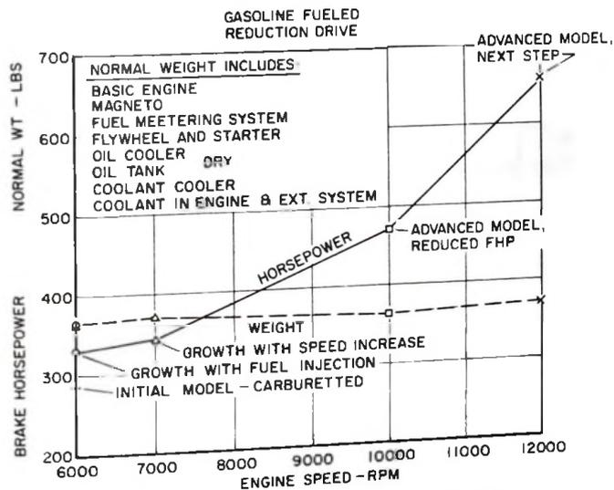
Figure 44. - RC2-75 output growth estimates, carbureted.
