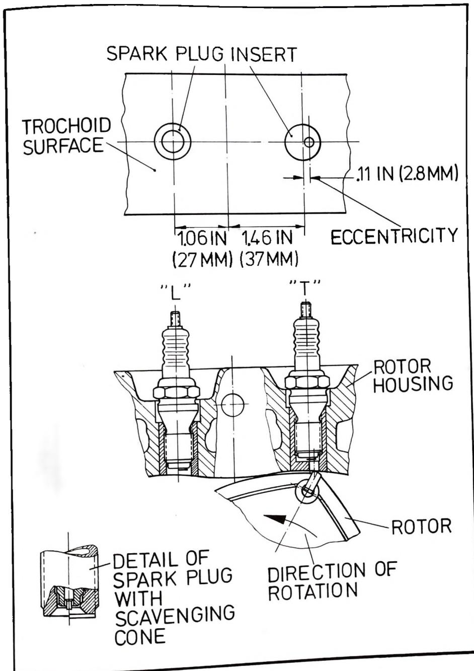
Figure 7. - Arrangement of spark plugs.
