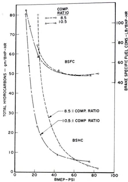
Figure 25. - Effect of compression ratio on fuel consumption and exhaust hydrocarbons.
