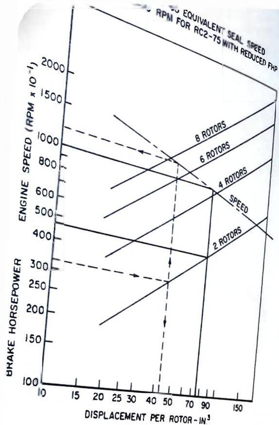
Figure 45. - Estimated RC engine power and speed.
