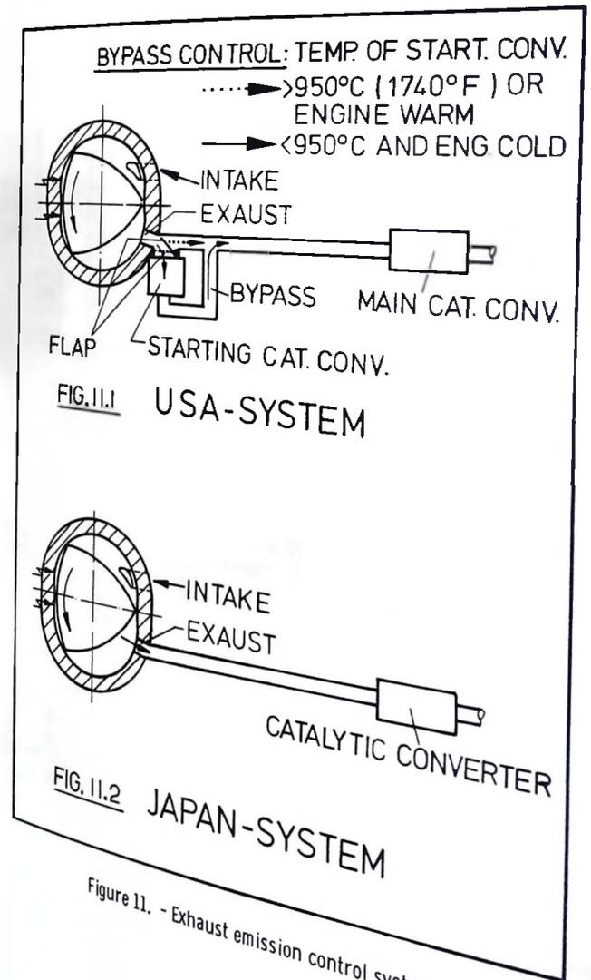
Figure 11. - Exhaust emission control system.
