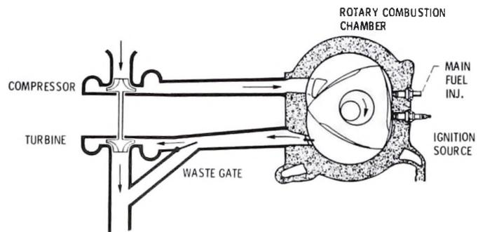
Figure 12. - Stratified charge rotary multi-fuel engine (conventional turbocharger).
