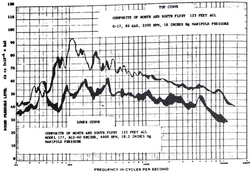
Figure 33 - Cessna 177 RC2-60 installation noise spectrum
