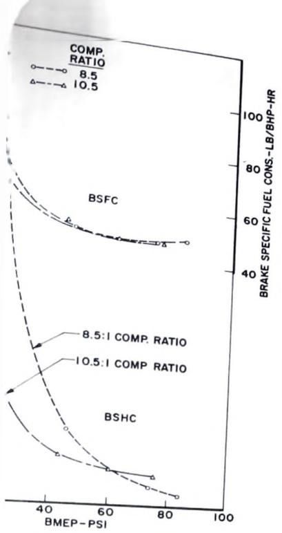
Effect of compression ratio on fuel consumption and hydrocarbons.
