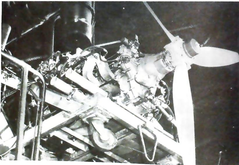
Figure 38. - RC2-75 engine on propeller test stand.
