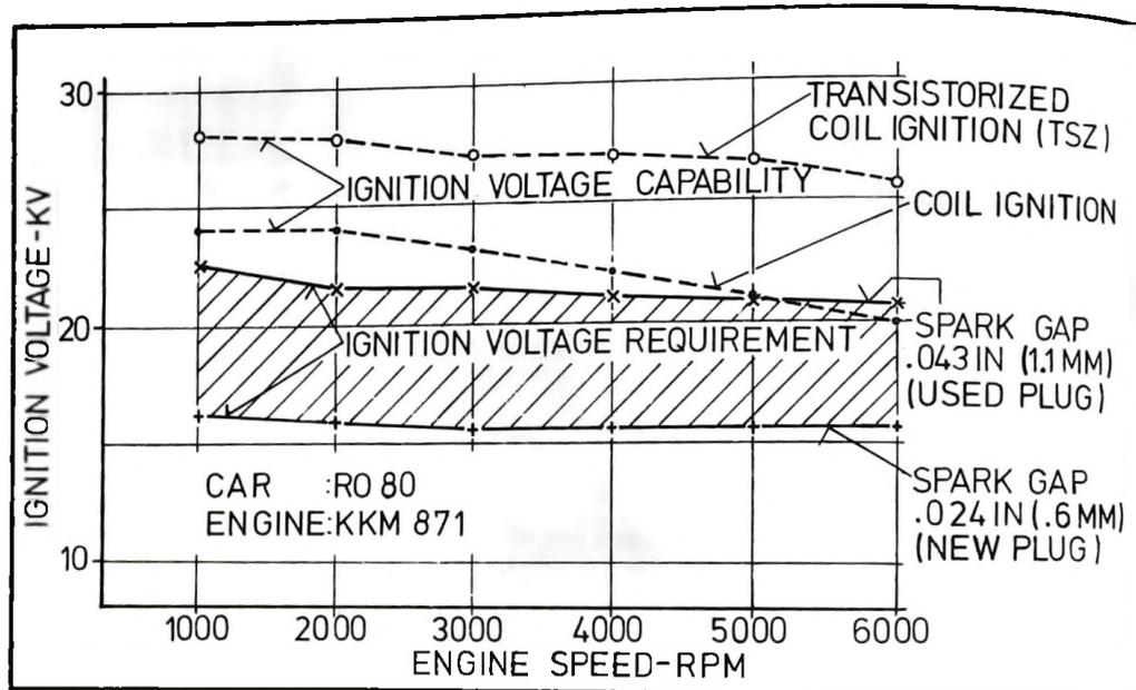
Figure 6. - Ignition voltage capability and requirement depending on ignition system and spark gap.
