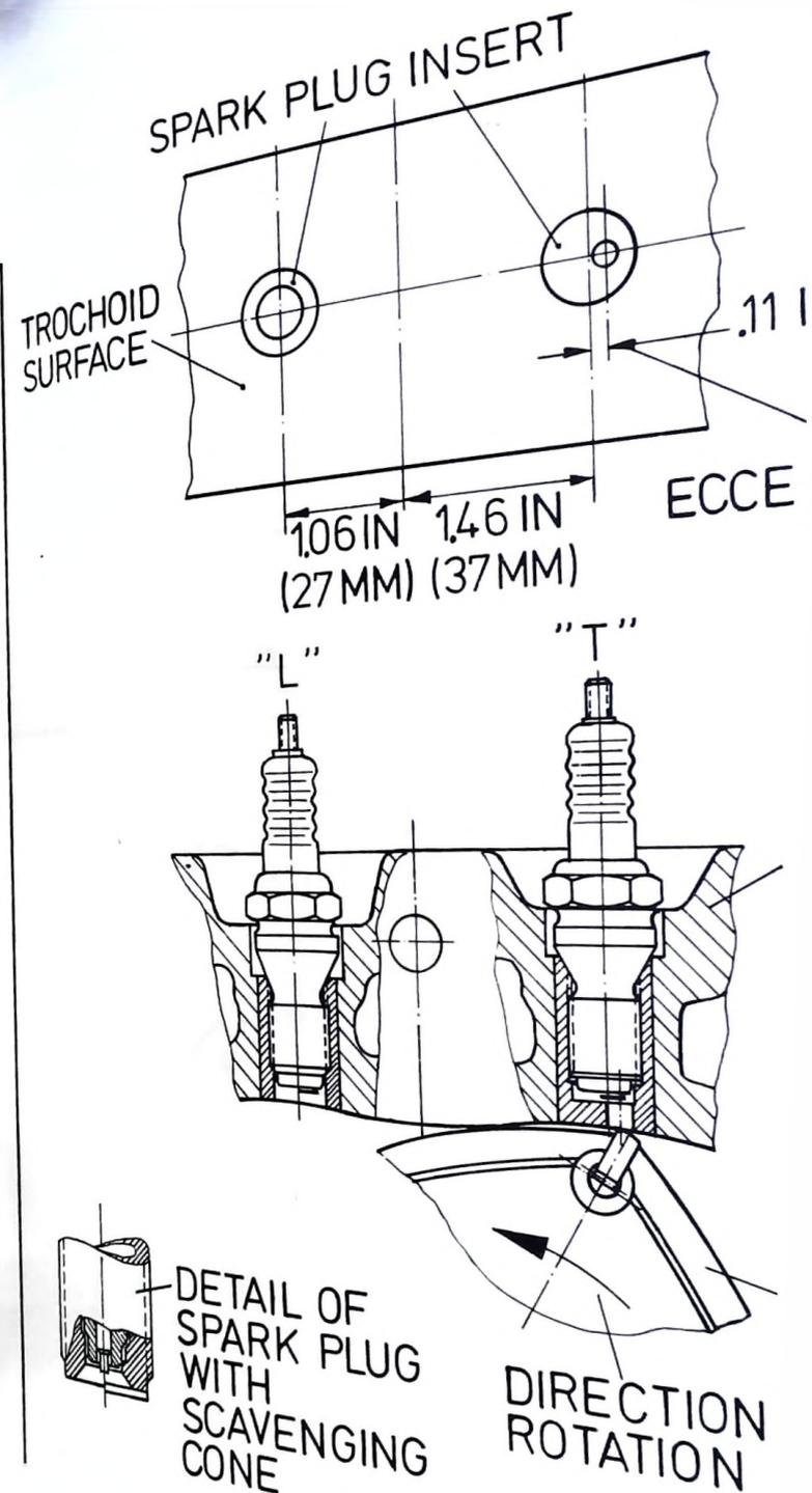
Figure 7. - Arrangement of spark plugs.
