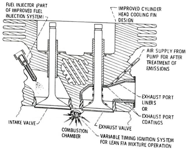
Figure 8. - Advanced cylinder head concept integration.
