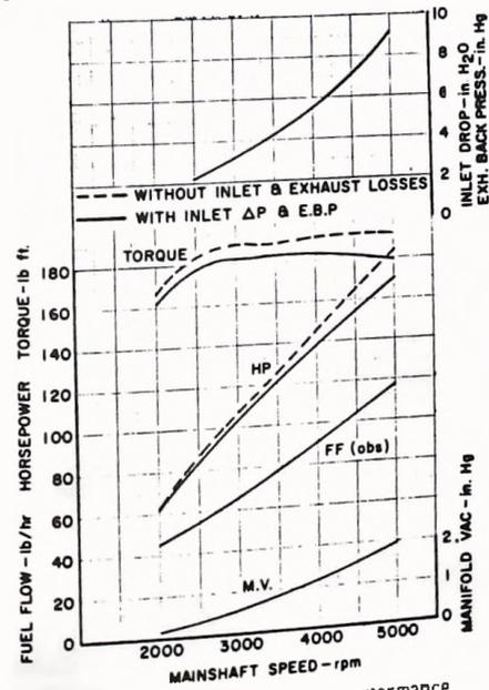
Figure 36. - RC2-60-Y8 test stand performance.
