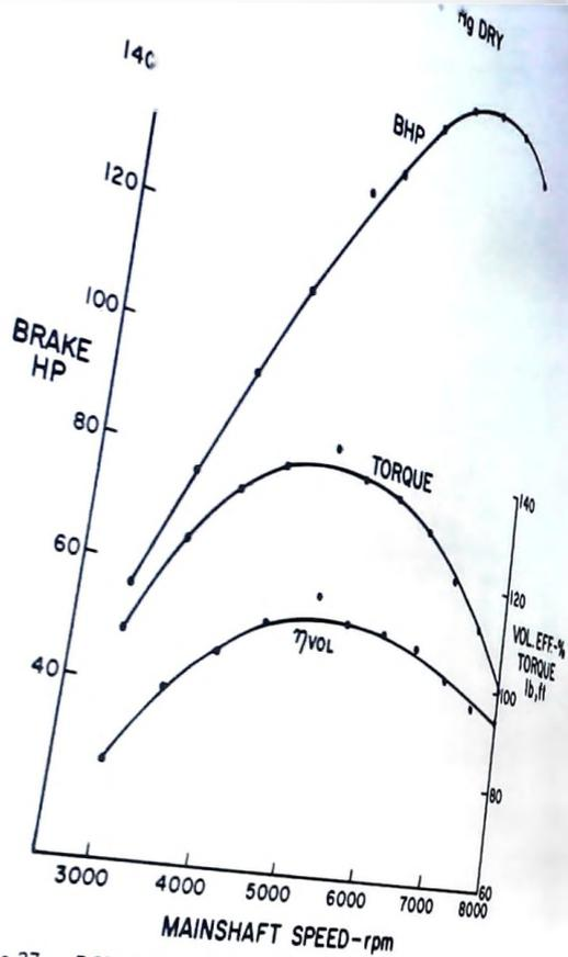
Figure 37. - RC1-60, peripheral port engine, performance at higher speeds.
