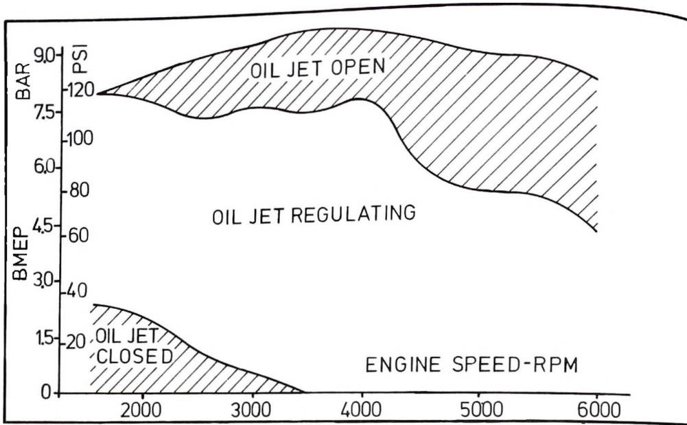
Figure 8. - Chart of oil jet control for rotor cooling.
