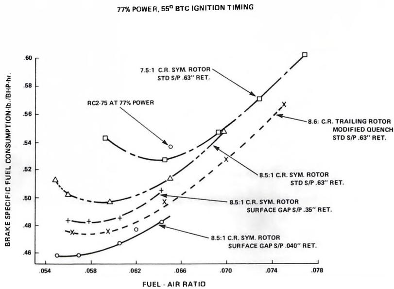
Figure 41. - RC1-75 cruise fuel consumption.
