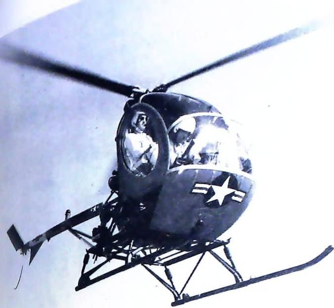
Figure 10. - Hughes helicopter with RC2-60 engine.
