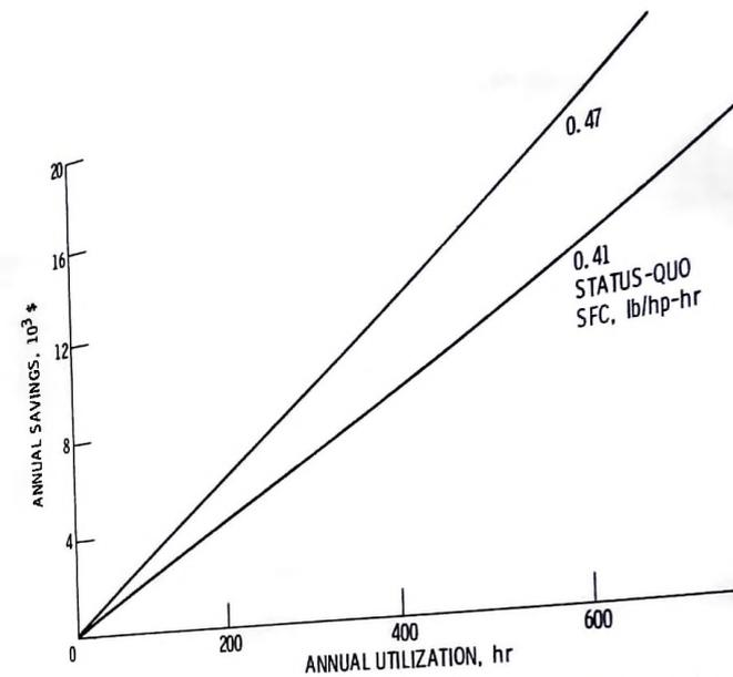
Figure 16. - Annual fuel cost savings due to advanced technology engine in 6-place twin.
