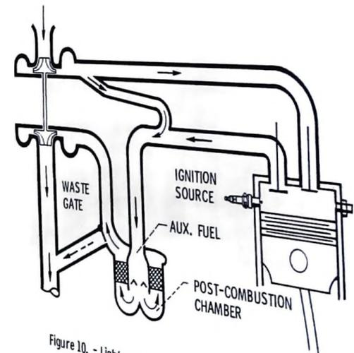
Figure 10. - Lightweight diesel or stratified-charge engine (semi-independent turbocharger).
