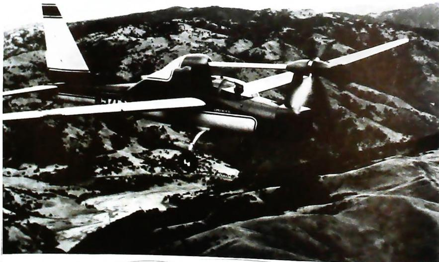
Figure 9. - Cessna Cardinal airplane with RC2-60 engine.
