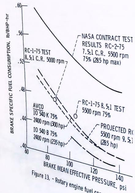
Figure 13. - Rotary engine fuel consumption trends
