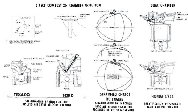
Figure 17. - Stratified charge processes.
