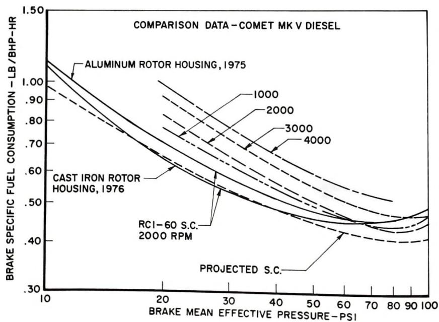
Figure 30. - Part load fuel consumption.
