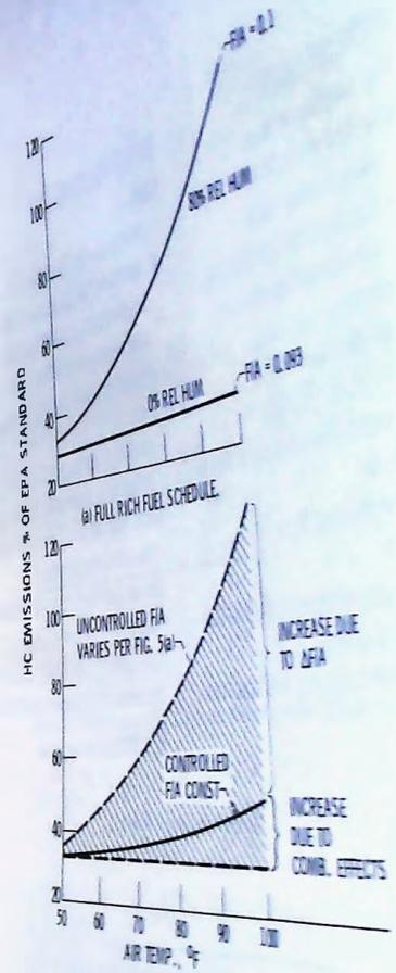
(b) EFFECT OF CONTROLLING FUEL/AIR RATIO TO CONSTANT VALUE AT 80% REL HUM.
