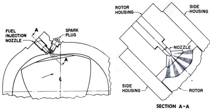
Figure 19. - Stratified charge RC engine, co-planar injection.
