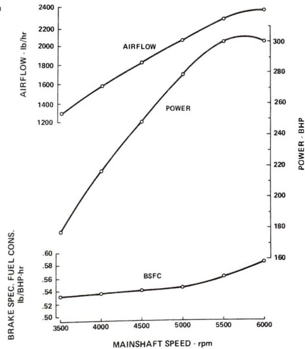
Figure 40. - RC2-75 full throttle performance, 7.5:1 compression ratio.
