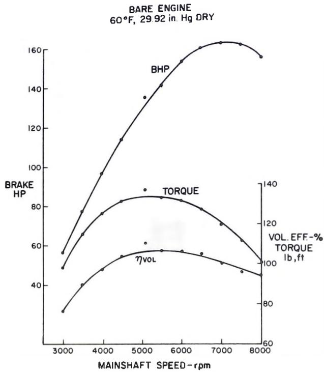
Figure 37. - RC1-60, peripheral port engine, performance at higher speeds.
