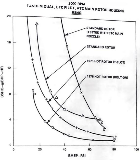
Figure 27. - Specific hydrocarbon emissions with standard and hot-insert rotors.
