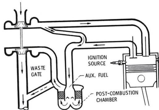
Figure 10. - Lightweight diesel or stratified-charge engine (semi-independent turbocharger).
