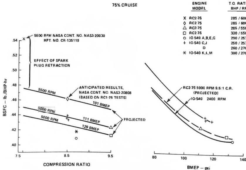
Figure 42. - RC2-75 cruise fuel consumption as function of engine compression ratio and rating.
