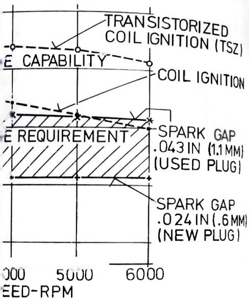
Ignition voltage capability depending on ignition system and spark gap.
