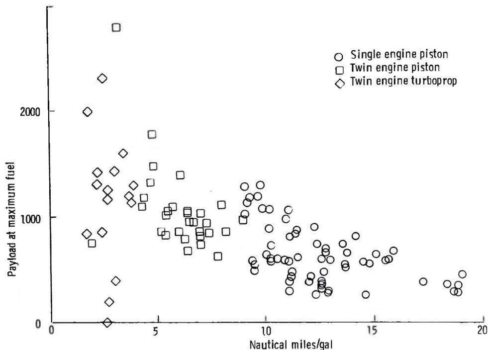
Figure 9. - Payload carrying efficiency for typical general aviation aircraft.
