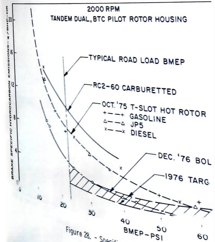
Figure 28. - Specific hydrocarbon emissions.
