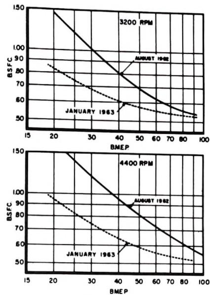
Figure 3. - SFC test results, January 1963, RC1-60.
