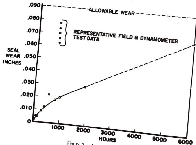
Figure 2. - Apex seal wear, RC2-60.
