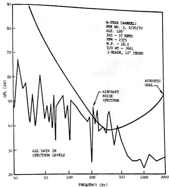
Figure 31. - Q-Star noise spectrum.
