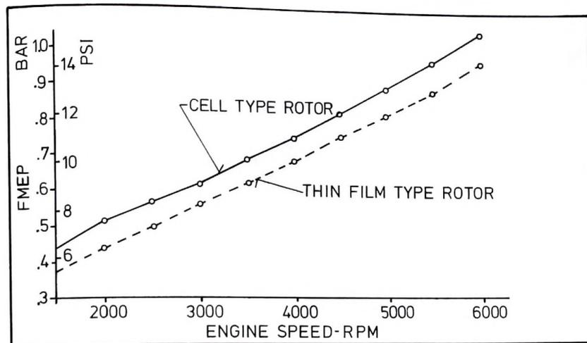
Figure 10. - Comparison of friction-MEP.
