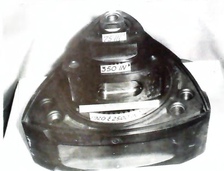
Figure 15. - Rotor comparison, 4.3 to 2500 cubic inch displacement.
