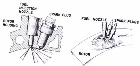
Figure 21 - Stratified charge RC engine showerhead injection.
