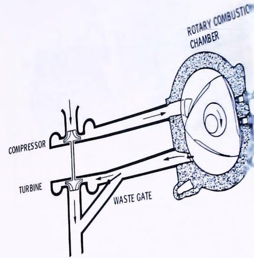
Figure 12. - Stratified charge rotary multi-fuel engine (conventional)
