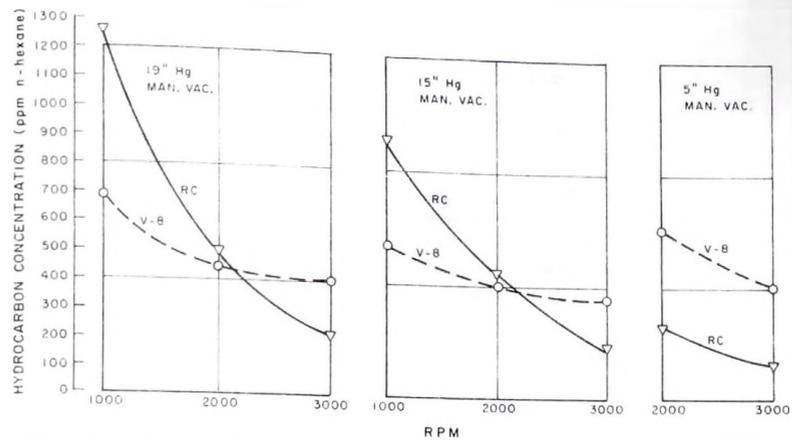
Figure 39. - RC2-60U5 and automotive V-8 engine raw emissions as function of engine speed.
