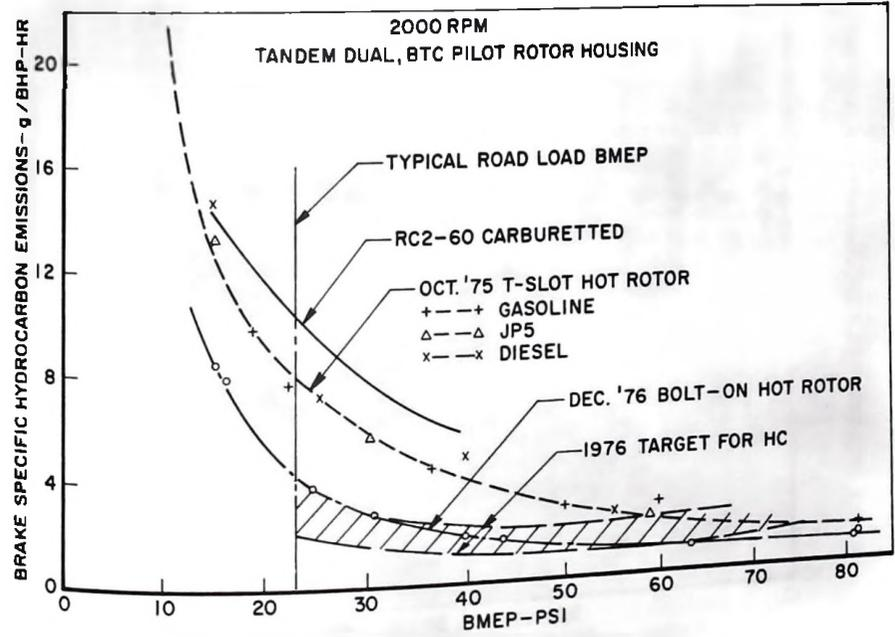
Figure 28. - Specific hydrocarbon emissions.
