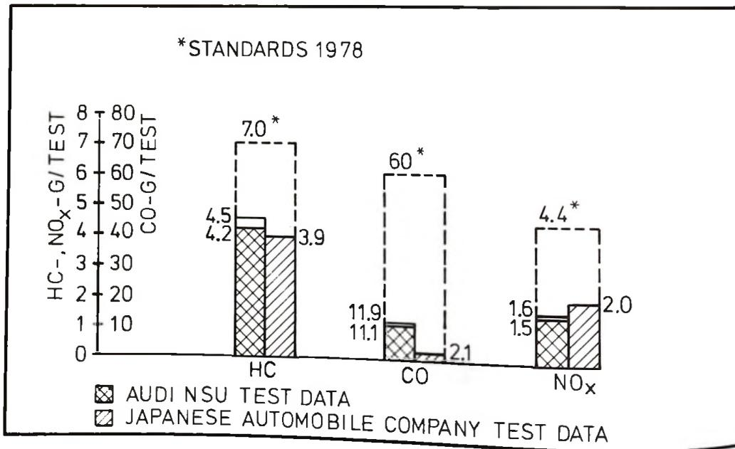
Figure 23. - Japanese 11-mode test exhaust emission data.
