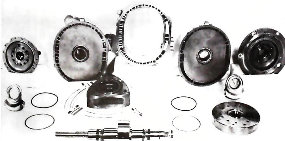
Figure 4. - Basic engine components, RC1-60.
