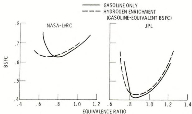
Figure 6. - Effect of hydrogen enrichment on fuel consumption.
