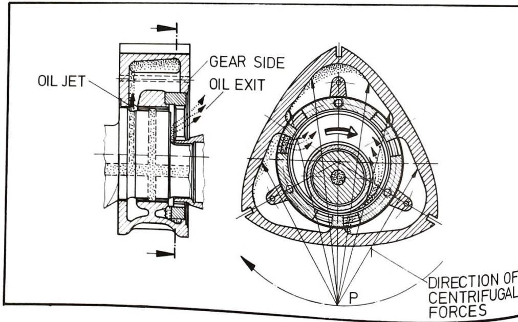
Figure 9. - Principle of cooling oil flow.
