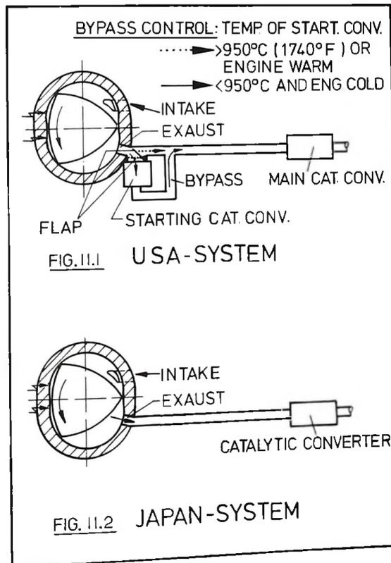
Figure 11. - Exhaust emission control system.
