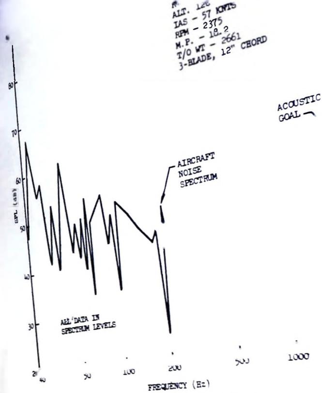
Figure 31. - Q-Star noise spectrum.
