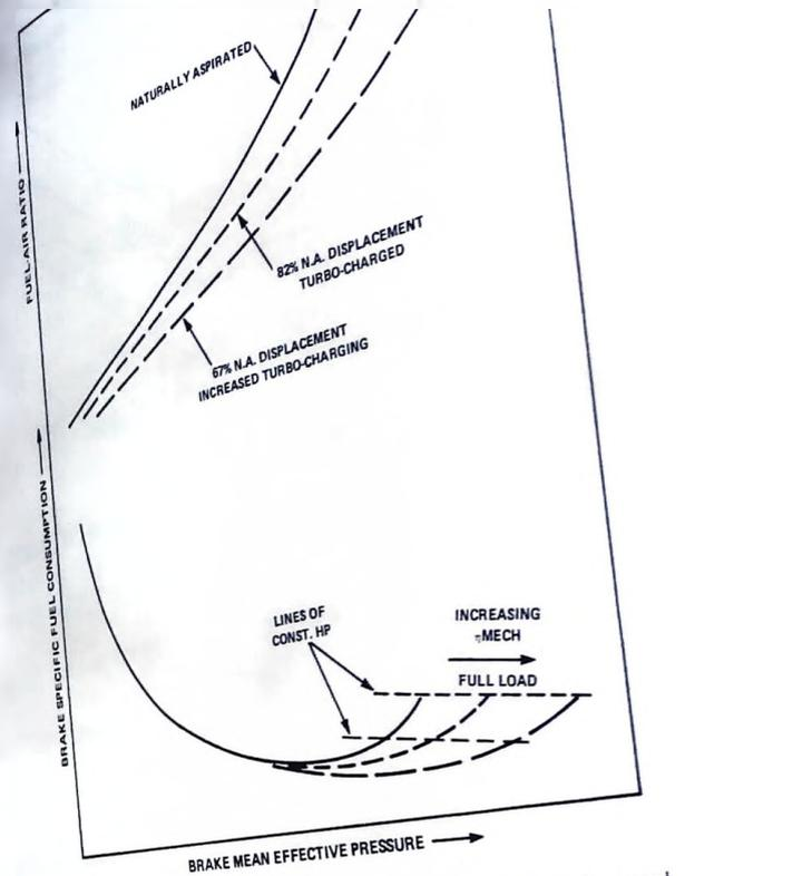
Figure 43. - Effects of decreasing stratified charge rotary engine displacement with corresponding increase in degree of turbocharging.
