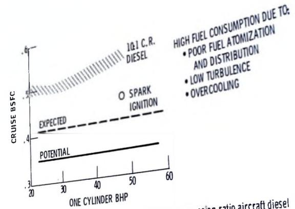
Figure 9. - Initial test results on cylinder low compression ratio aircraft diesel at the University of Michigan.
