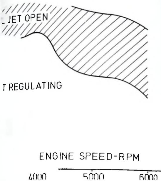
part of oil jet control for rotor cooling.
