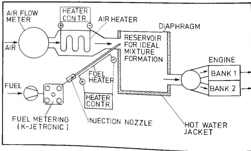
Figure 13. - Arrangement of ideal mixture formation system.
