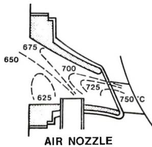
ENGINE:13B 1500 RPM BMEP:1KG/CM<sup>2</sup>
