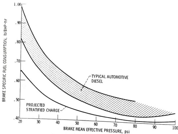
Figure 15. - Rotary engine fuel consumption trends.
