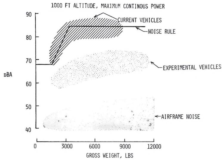
Figure 5. - Noise levels of small propeller driven vehicles.
