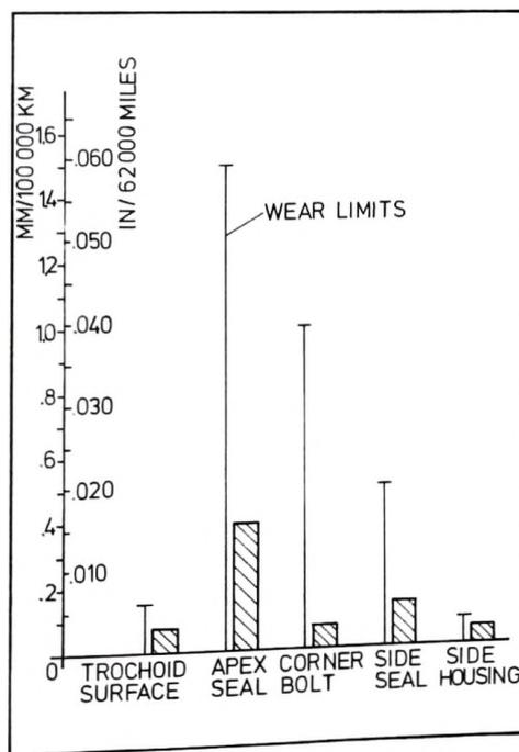
Figure 25. - Average wear data of durability tests.
