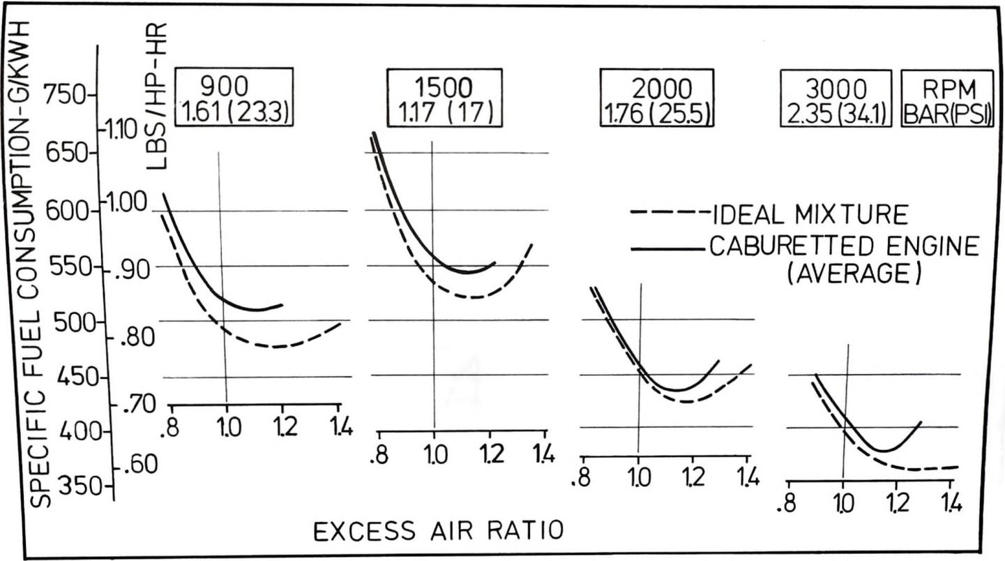
Figure 14. - SFC at part load of R. E. with ideal mixture.
