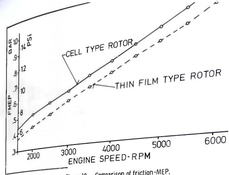
Figure 10. - Comparison of friction-MEP.
