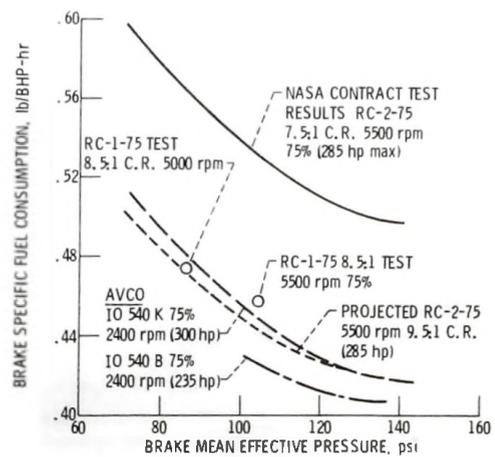
Figure 13. - Rotary engine fuel consumption trends.
