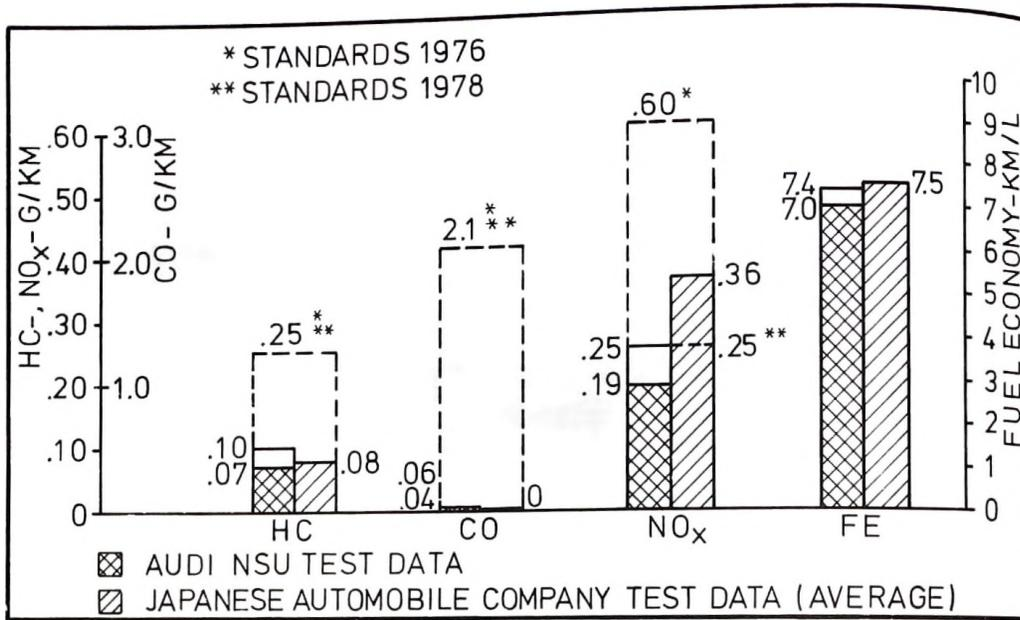
Figure 22. - Japanese 10-mode test exhaust emission data and fuel economy.
