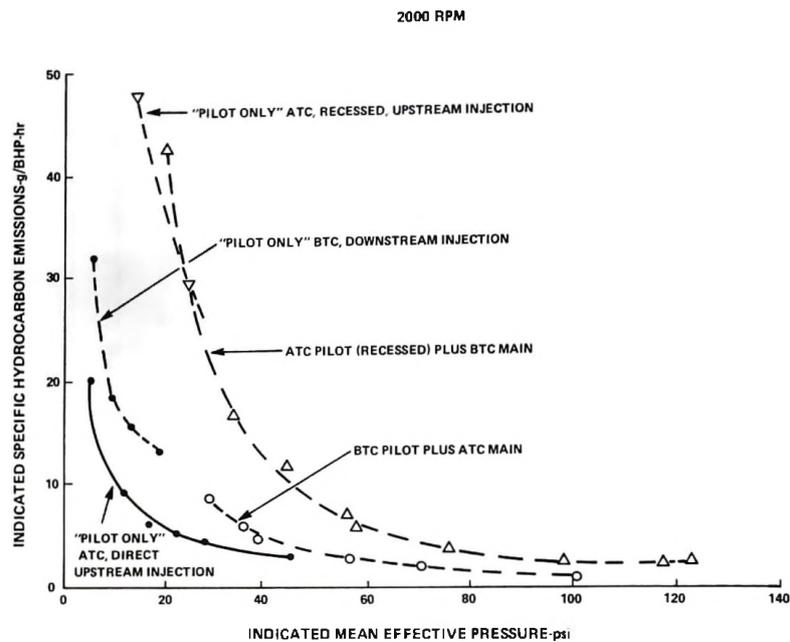
Figure 29. - Indicated specific hydrocarbon emissions comparison of different pilot locations.
