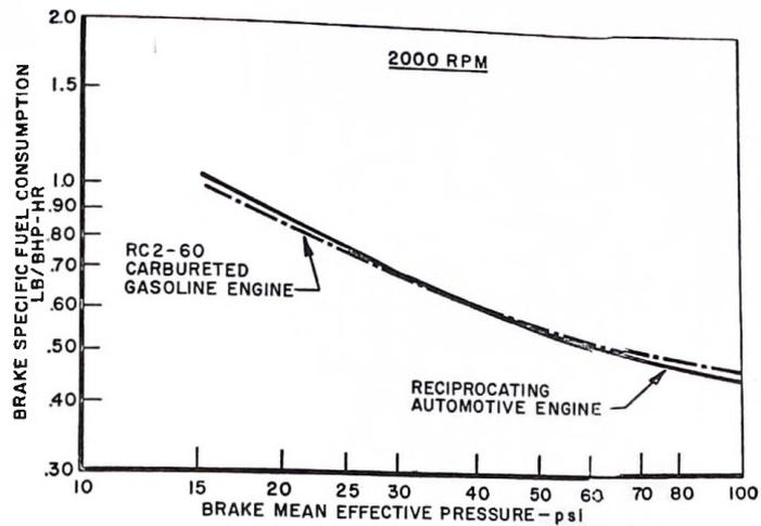
Figure 6. - RC2-60 part load fuel consumption.
